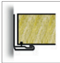
Clip-on profile to conceal rivets upon request.
